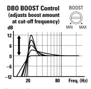
Figure 13. Frequency response curves show typical DBO control ranges for the JBL A6000GTi or A3000GTi amplifier.
